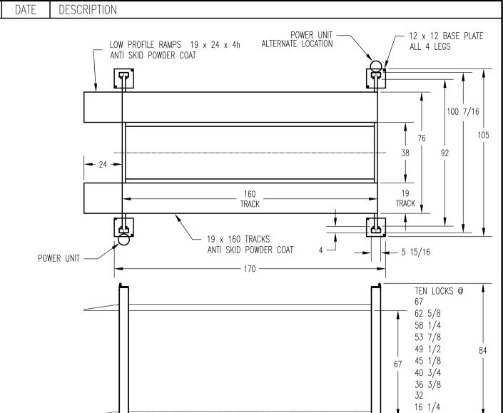
CAPACITY 7000lbs 110v 1 hp 30 amp single phase OR - 220v 2 hp 30 amp single phase POWDER COAT FINISH, WHEEL STOPS, 10 LOCKING POSITIONS FOR VERSATILITY AND SAFETY
