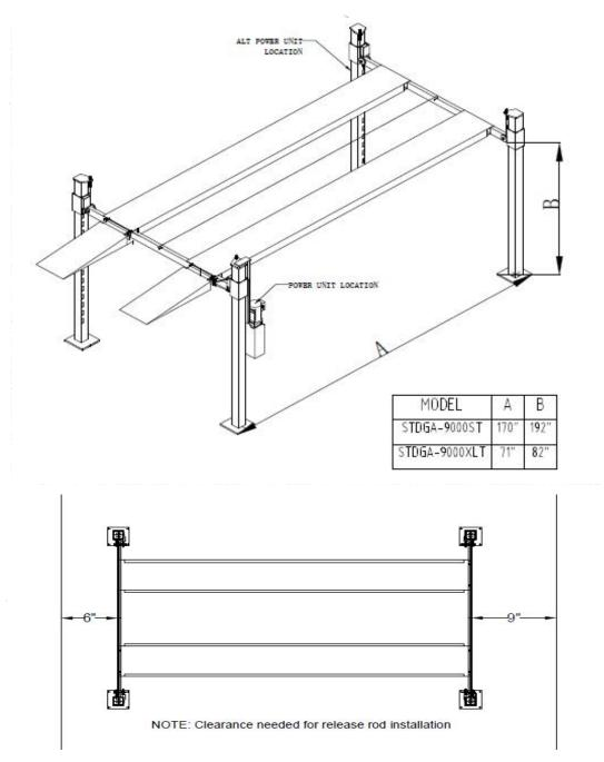
3. Make a chalk line layout of the lift following the dimensions listed (see fig. 1). **IMPORTANT NOTE:** Follow clearance requirements listed (see fig. 2)
