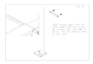
7 Place the offside runway on the cross tubes. Repeat steps 3-6 for the offside runway. Do not tighten bolts until lift instiallation is complete.
